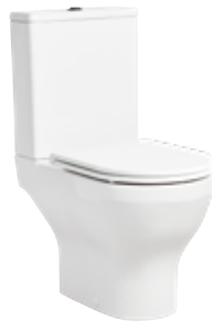
Open Back Close Coupled WC Spigot distance from wall 140mm 365(w) x 852(h) x 620(d)mm
