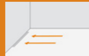
Drain positioned against the short wall
