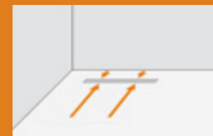
Drain positioned off the wall
