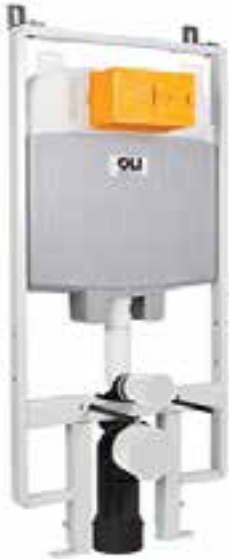
1200cm Slim Pre-wall, freestanding w.c frame including brackets and w.c bend with 3/6 litre dual flush plate front flush installation only.
